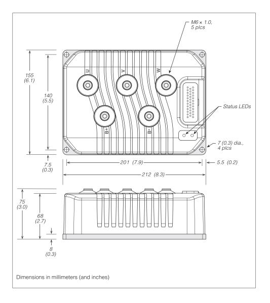
heatsink to the mounting surface. Additional heatsinking or fan cooling may be necessary to meet the desired continuous ratings.
