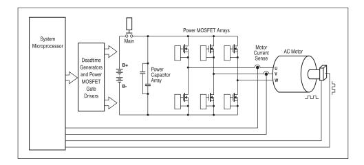
Heavy copper busbars connect the IMS modules to the brass external motor connection studs. A bank of power capacitors keeps DC bus levels stable during high frequency MOSFET switching and also reduces EMI on the external B+ and B- cables.
