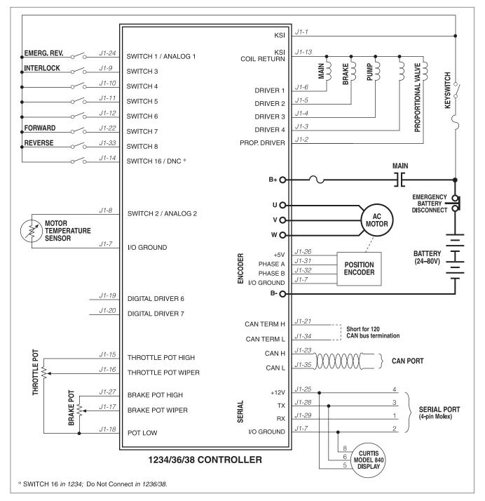
Fig. 3 Basic wiring diagram, Curtis 1234/36/38 motor controller.
