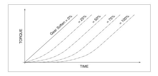
**Fig. 10** Effect of Brake Taper Speed parameter (torque control mode).
