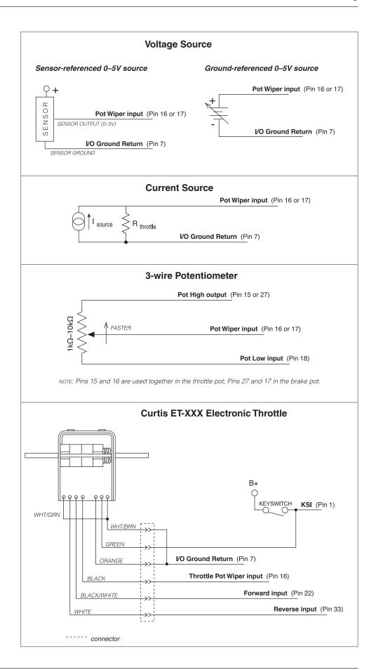
When a 3-wire potentiometer is used, the controller provides full fault protection in accordance with EEC requirements. The pot is used in its voltage divider mode, with the controller providing the voltage source and return. Pot High provides a current limited 5V source to the pot, and Pot Low provides the return path. This is the throttle shown in the basic wiring diagram (Figure 3) for the drive throttle and for the brake throttle.
