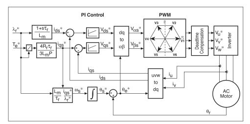
The controller uses an advanced pulse width modulation technique to maximize the utilization of battery voltage, minimize harmonic losses, and increase system efficiency. This method achieves 15% greater linear utilization of battery voltage, thereby effectively getting more usable motor power than standard PWM at the same battery voltage.
